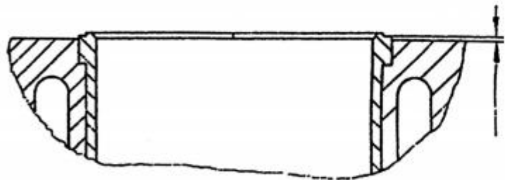
Fig.6 Protruding height of the liner flange plane relative to the plane of cylinder block
